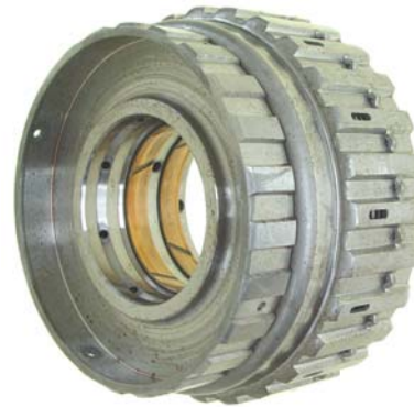
Direct clutch drum
