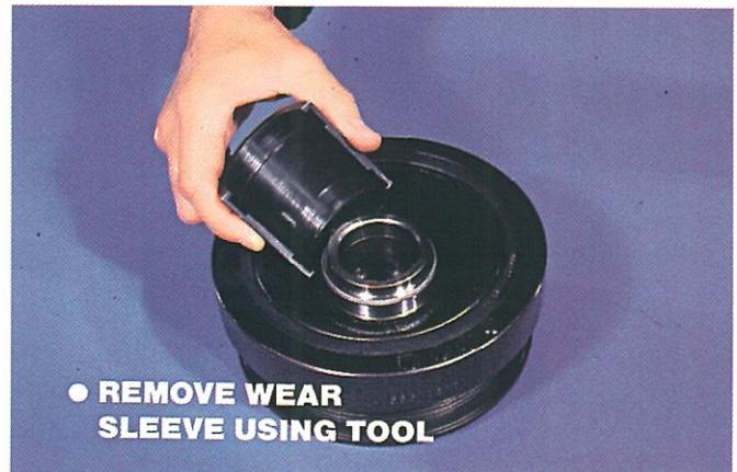
● REMOVE WEAR SLEEVE USING TOOL
