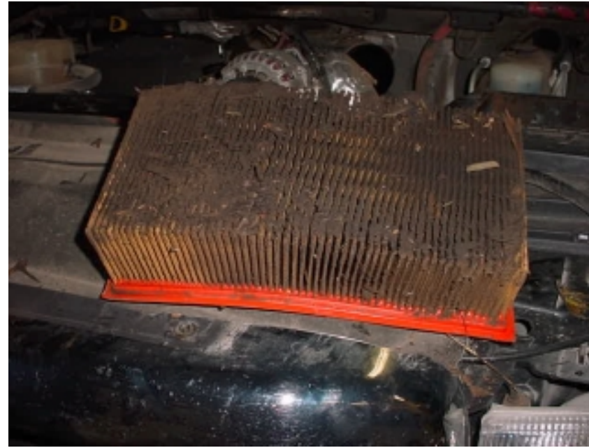
Example of Excessive Debris in Air Filter
