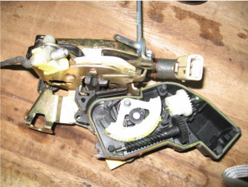
Prying the two tabs open on the motor
