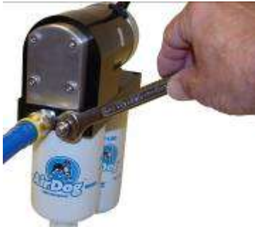
Loosen the Jam Nut Re-Torque After Adjusting
