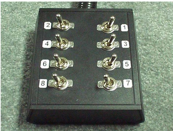
I started at the box, drilling 8 holes for the switches, arranged like each bank of cylinders I drilled the holes a bit undersized, then carved a post in them to match the notch in the switch. This helps hold them in the correct position. I arranged my switches so they were off toward the center of the box on both sides. I connected ring terminals to one end of 8 ft pieces of wire, one red and one black for each wire. I found it's easiest to fasten the terminals on
