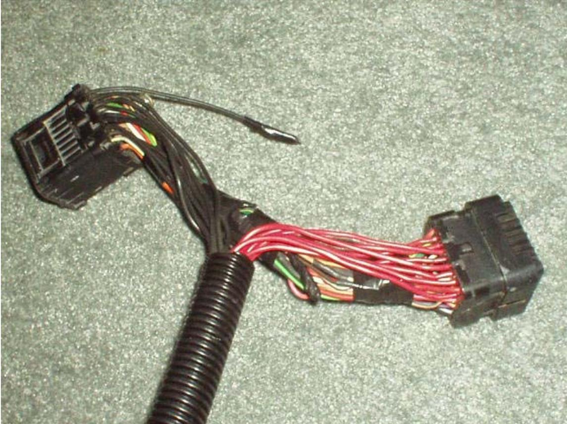
This photo shows the final arrangement of the plugs on my tester. Pins 2-8 and 10 (red and black wires in the photo) are the injector circuits, which I wired last. All the other pins connect to their corresponding number in each connector half (numbers are on the back). My female connectors didn't have enough pins to fill all the holes, but they're not all used on the PSD.
