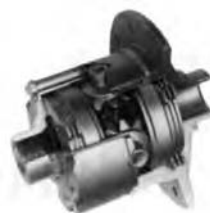
POWR-LOK™ 2-Piece Case 4 Pinion Mate Gears
