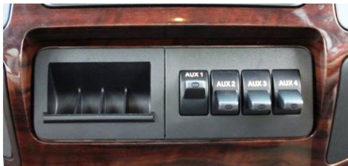
Finished installation of Upfitter Switches without Trailer Brake Controller (Coin Slot)
